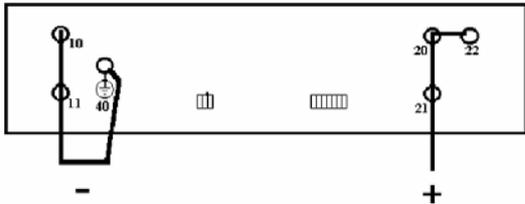
Figure 6. Output to case isolation voltage test.
