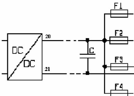
Figure 2. Connecting multiple loads.
