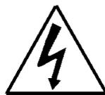
The lightning flash with arrowhead, within an equilateral triangle, is intended to alert the user to presence of uninsulated "dangerous voltage" within the products enclosure that may be of sufficient magnitude to constitute a risk of electric shock to persons
