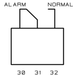
Figure 3. Alarm contact.
